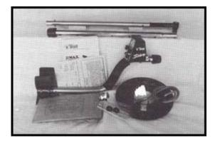
Assembly of the CUTLASS II  $\mu$ MAX is simple and requires no special tools. Just install the battery, mount the searchcoil on the lower pole assembly, connect the two pole assemblies together, wrap the excess cable around the pole and plug the cable into the control housing. Finally, adjust the pole length and searchcoil angle and you're ready!
