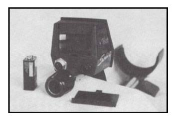
To install or replace the battery, first make sure the SENSITIVITY control is set to POWER OFF—turned completely counterclockwise past the "click." Remove the battery door from the back of the control housing. Do this by pressing your thumb firmly on the louvered square—at the bottom of the battery door—and sliding the battery door upward (in the direction of the arrow) while pushing.
