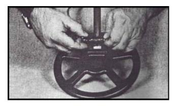
Note: The pole tip should fit very snugly into the mounting ears.
