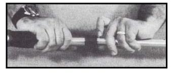
Note: The plastic lock nuts will be used to eliminate any "slop" in the pole joint by turning it counterclockwise to the locked position.
