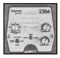
This may cause your detector to become unstable and force you to turn the SENSITIVITY knob to a lower setting. An overload situation will not hurt your detector, but it will maximize the gain that is used by your detector. This can, in certain conditions such as low mineralization in the soil, cause your detector to penetrate deeper into the ground and become more sensitive to small targets.
