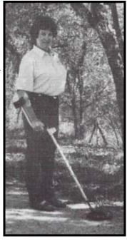
To adjust the searchcoil angle, simply loosen the searchcoil thumb nut slightly and move the searchcoil into the desired position. Tighten the searchcoil thumb nut by hand so that the searchcoil will hold in place.
