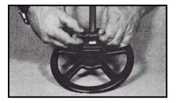
Note: The pole tip should fit very snugly into the mounting ears.
