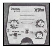
Changing the operating frequency will not change the audio frequency of the signal in the speaker. The audio frequency is controlled by a microprocessor and will not shift.
