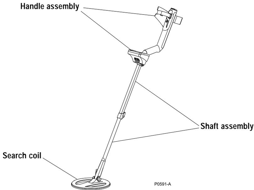
Please follow these instructions to assemble the Explorer II. Refer to the drawings to identify parts and how they are positioned. The detector's components are organized into three categories:
