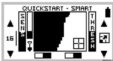
Figure 5.3 Smartfind display with preset Coins discrimination pattern
