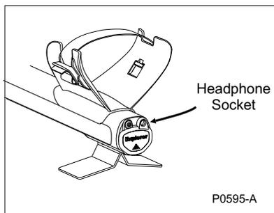
Figure 2.14 Inserting headphone
